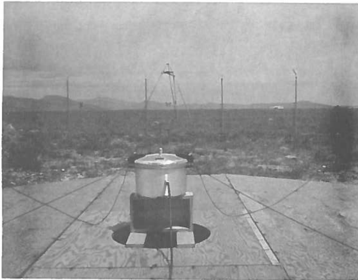
Figure 8. Monopole antennas at site Ra for Test No.
