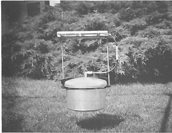
Figure 9. Horizontal dipole and transmitter assembly.
